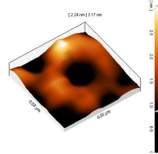
Fig. 3: three dimension (3D) AFM images of ZnS/glass thin layer
