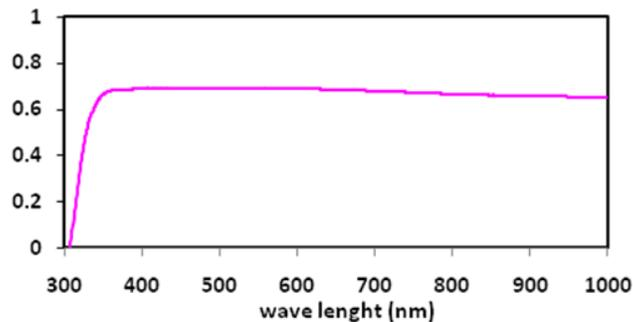
Fig. 7: Transmittance diagram of ZnS/glass thin layer.
