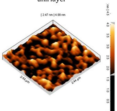
Fig 2: three dimension (3D) AFM images of ZnS/glass thin layer
