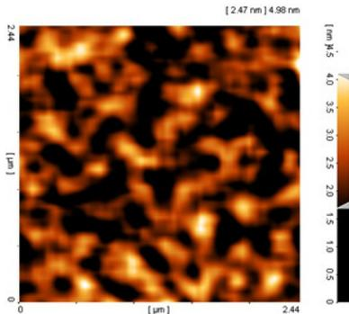
Fig. 1: two dimension (2D) AFM images of ZnS/ glass thin layer
