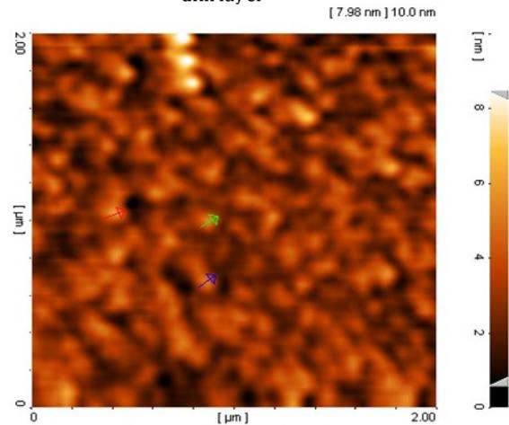
Fig. 4: two dimension (2D) AFM images of ZnS/ glass thin layer
