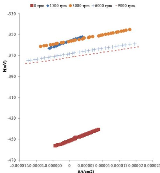
Fig. 1: the curves obtained from linear polarization tests C95700 alloy for different speeds of rotation samples in 3.5% sodium chloride solution at room temperature.
