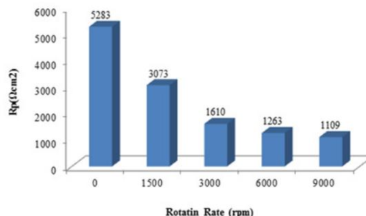
Fig.9: The changing polarization resistance at different rotation speed at 40 ° C
