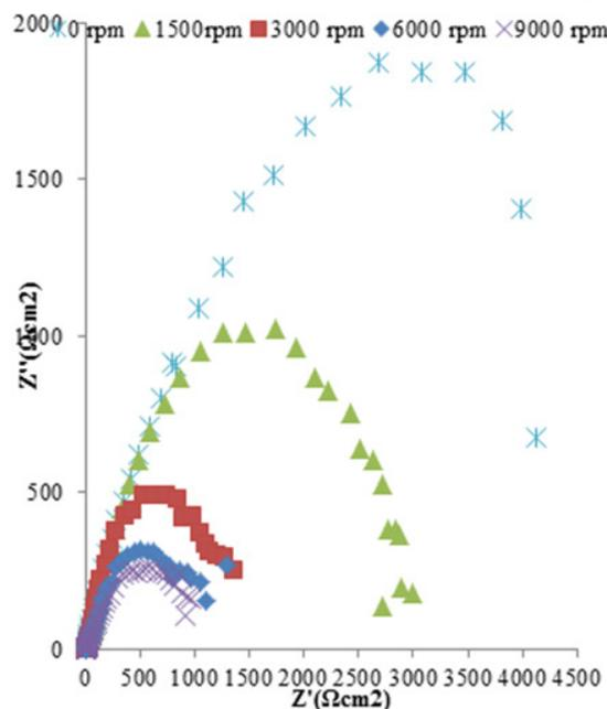
Fig.8: The electrochemical Nyquist curves of C95700 alloy at different rotation speeds of the sample in 3.5% sodium chloride solution at room temperature.
