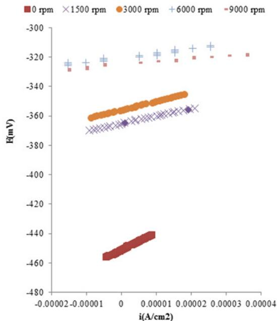
**Fig. 5:** The curves obtained from linear polarization tests of C95700 alloy at different rotation speed of the sample in 3.5% sodium chloride solution at 40 ° C
