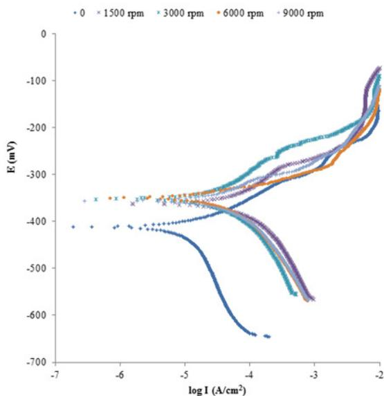
**Fig. 3:** The electrochemical polarization curves at different rotation speeds of C95700 alloy sample in a solution of 3.5% sodium chloride at room temperature
