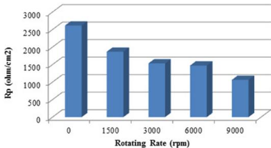
Fig. 6: The variation polarization resistance of C95700 alloy at the different rotation speed at 40 ° C
