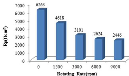
Fig. 2: the changes polarization resistance of the C95700 sample in sodium chloride solution or different speeds of rotation samples in 3.5% sodium chloride solution based on linear polarization testing at room temperature.
