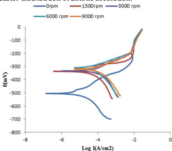
Fig. 7: The electrochemical polarization curves at different rotation speeds of the samples in 3.5% sodium chloride solution at 40 ° C
