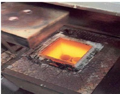
**Fig. 9:** Underground furnaces for melting Al & SiC
