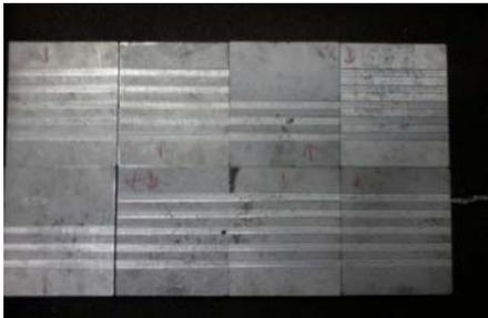
Fig. 16: End Milled (Slot) Al 2024-SiC plates
