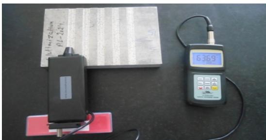
Fig. 18: ITI SurfTest to measure Surface roughness
