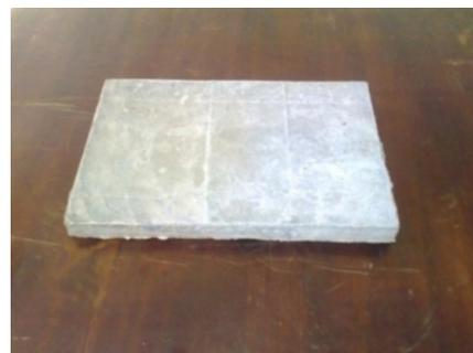
**Fig. 7:** Stir Cast Plate of Al 2024 -SiC Composite
