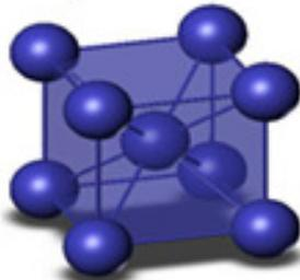
Fig. 2: The simplified diagram of BCC crystal lattice
