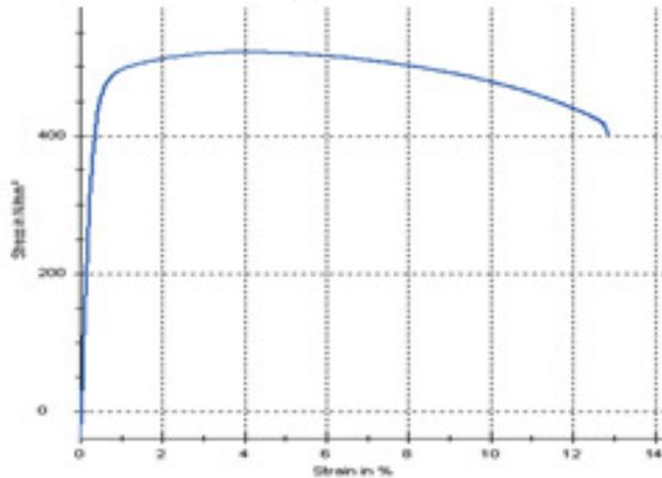
Fig 7: Strain-stress curve of cold rolling section of structural steel
