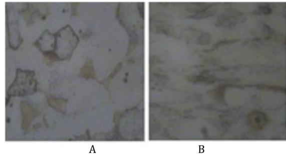
Fig 5: Metallography picture from Sample A, B: sample A produced by normal structural steel, sample B produced by cold formed structural steel
