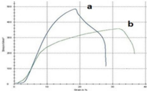
**Fig. 11:** Stress-strain curves (a: Cold rolling condition, b: Normal condition)
