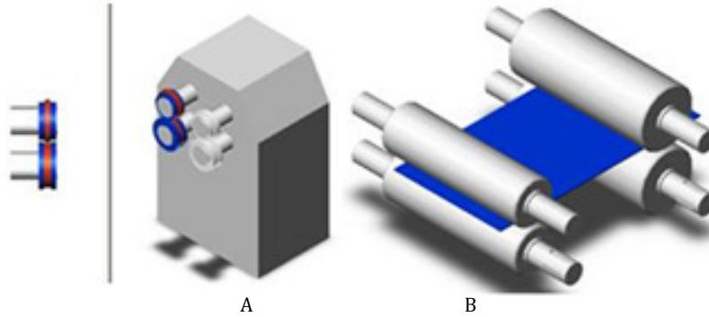
Fig. 1: Two applicable procedure in cold forming process (A: for sections, B: for sheets)
