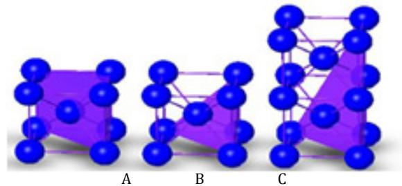
Fig. 3: Slipping plan in BCC crystal structure: A. plane (110), B. plane (111), C. plane (112)
