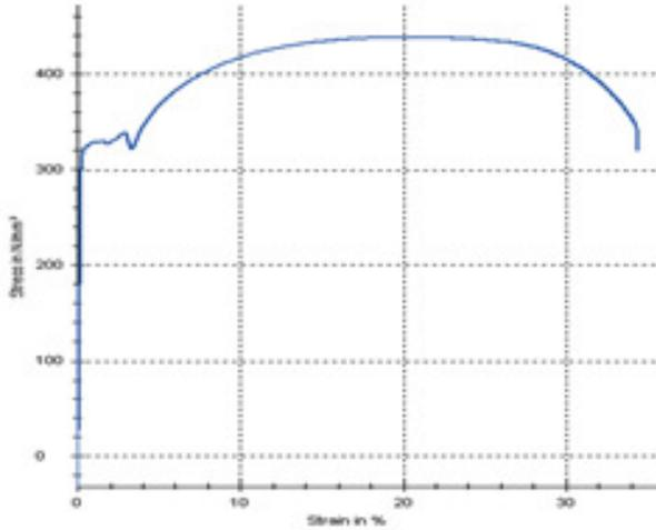
Fig6: Strain-stress curve of normal section of structural steel
