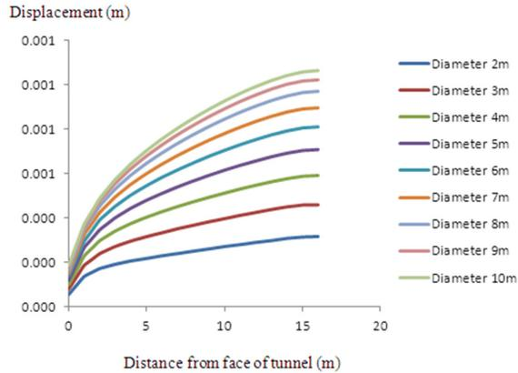
**Fig. 4:** The values of displacement around the cylindrical tunnels for different distances from tunnels face ( $K_0=1.2$ )
