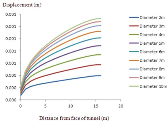
**Fig. 5:** The values of displacement around the cylindrical tunnels for different distances from tunnels face ( $K_0=1.5$ )
