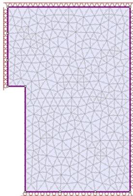
Fig. 1: Modeling of the cylindrical tunnel with diameter 2 meters for axisymmetric analysis
