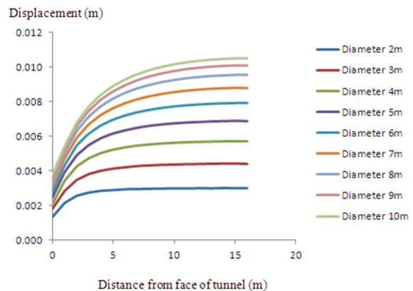
Fig. 3: The values of displacement around the cylindrical tunnels for different distances from tunnels face
