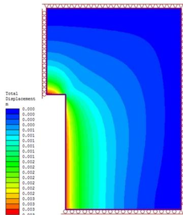
Fig. 2: Total displacements in around the cylindrical tunnel with diameter 2 meters
