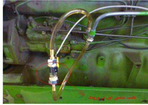
**Fig. 10:** Injector pump water mill JD 3140 and the place of the entrance of the fuel to the pump
