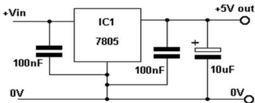
Fig. 2: Schematic view of the power supply
