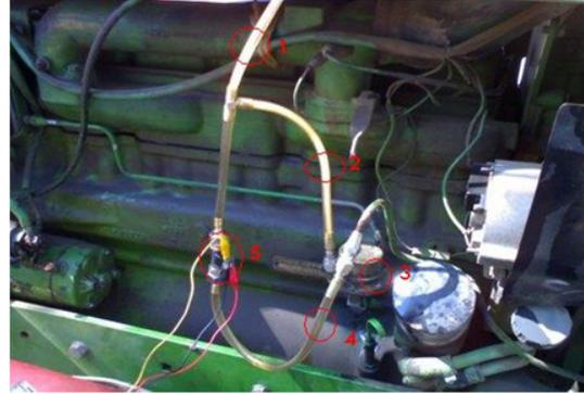
**Fig. 11:** The location of the sensor flow meter at the entrance of the fuel to the injector pump
