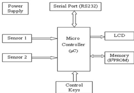
Fig. 1: Overview of the components used in the fuel measurement system
