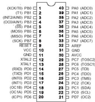
Fig.6: Atmega16 microcontroller
