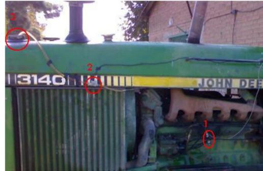
**Fig. 12:** The location of fuel flow meter sensor in the input and output of the fuel, 1- Sensors measure the amount of fuel input, 2- sensors measure the amount of fuel 3- Unloading the fuel tank as measured by the tractor
