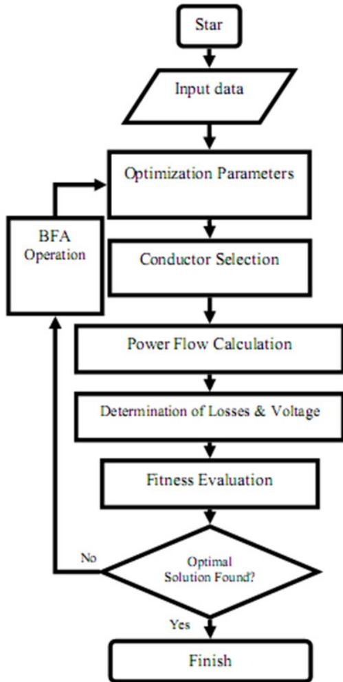
Fig.2: Flowchart of the proposed BFA algorithm
