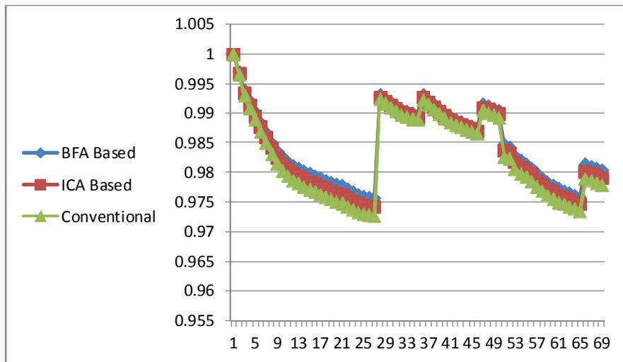
**Fig.6:** Voltage profiles of 69-bus system
