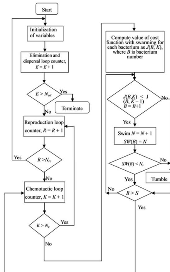
Fig.4: Flowchart of the proposed BFA algorithm
