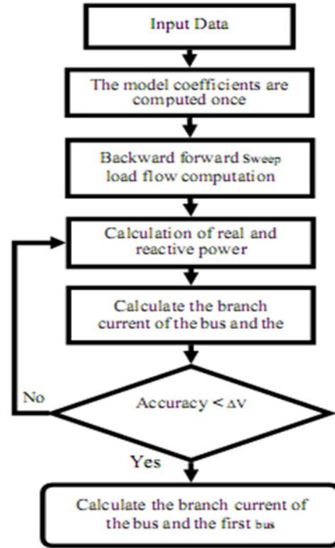
Fig.1: Flowchart of the Backward-Forward sweep method
