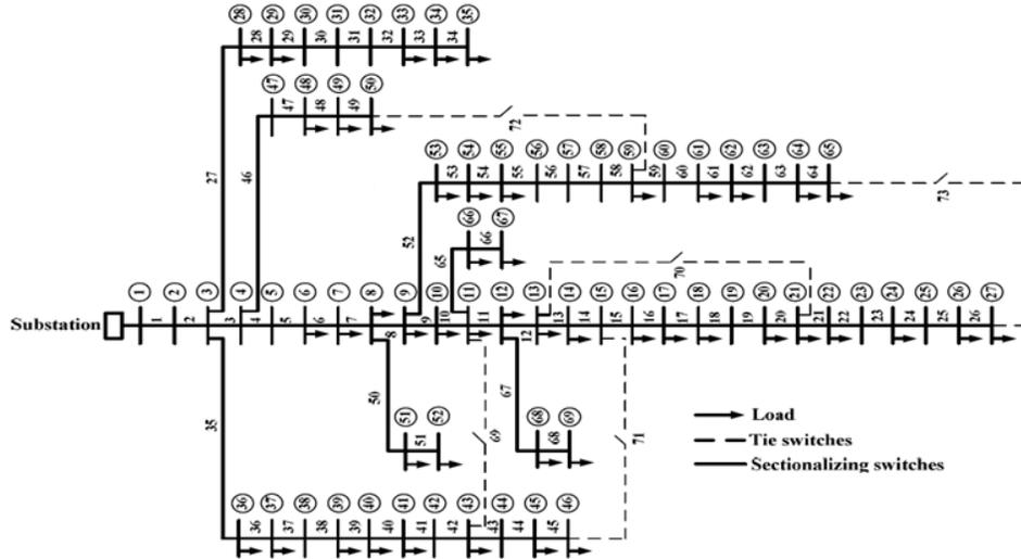
Fig.5: Single line diagram for a 69-bus radial distribution system
