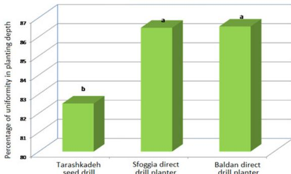
Fig.3: Comparing the mean percentage of uniformity in planting depth by the seed drills
