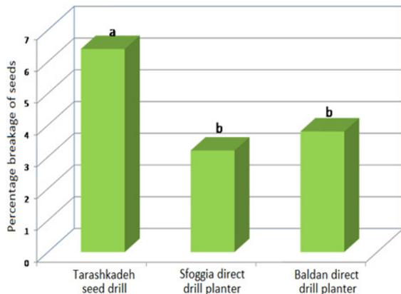
**Fig.1:** Comparing the means of percentage breakage of seeds in the seed drills
