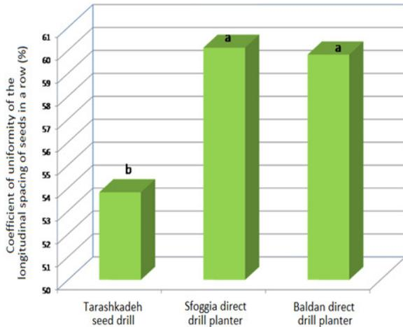
Fig.2: Comparing the accuracy of the drills in providing uniform suitable spacing between the seeds in rows
