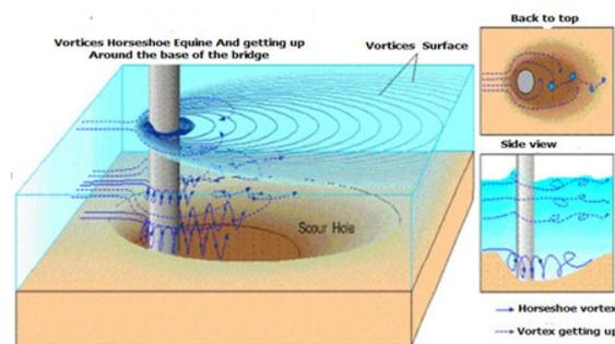
Fig.2: Mechanism of formation of horse shoe vortices sand vortices getting up
