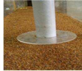
Fig.4: basic model of the bridge with a protective collar around its
