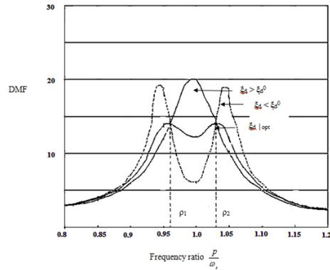
Fig. 3: Response curve for amplitude of system with optimally tuned TMD
