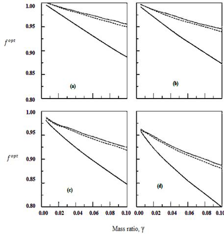
**Fig. 7:** Variation of the optimum tuning frequency ratio versus mass ratio for,  $f = f^{opt}$ ,  $\beta = \beta^{opt}$  and  $\xi_T = \xi_T^{opt}$  (a)  $\xi_s = 0\%$  (b)  $\xi_s = 2\%$  (c)  $\xi_s = 5\%$  (d)  $\xi_s = 10\%$   $n = 1, \dots, n = 11, \dots, n = 21$ .
