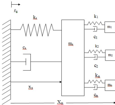
Fig. 4: A multiple tuned mass damper system
