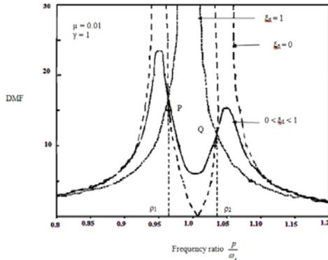
Fig. 2: Amplitude of main mass for various values of absorber damping.
