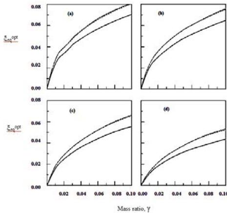
**Fig. 8:** Variation of the optimum equivalent damping ratio versus mass ratio, for  $f = f^{opt}$ ,  $\beta = \beta^{opt}$  and  $\xi_T = \xi_T^{opt}$  (a)  $\xi_s = 0\%$  (b)  $\xi_s = 2\%$  (c)  $\xi_s = 5\%$  (d)  $\xi_s = 10\%$ .
