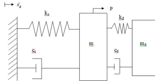
Fig. 2: Undamped SDOF system coupled with damped TMD system
