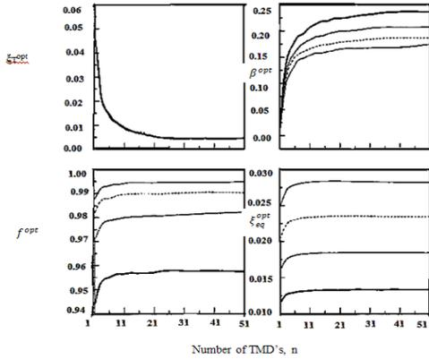
**Fig. 5:** Variation of the optimum parameters versus no. of tuned mass damper, for  $\gamma=1\%$  and  $\xi_s=0, 2, 5, 10\%$ .
