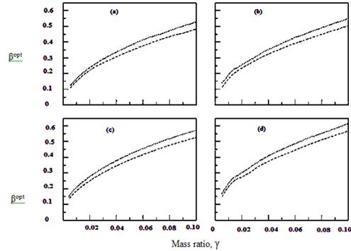
**Fig. 6:** Variation of the optimum frequency range of the MTMD versus mass ratio, for  $f=f^{opt}$ ,  $\beta=\beta^{opt}$  and  $\xi_T=\xi_T^{opt}$  (a)  $\xi_s=0\%$  (b)  $\xi_s=2\%$  (c)  $\xi_s=5\%$  (d)  $\xi_s=10\%$   $n=1, \dots, n=11, \dots, n=21$
