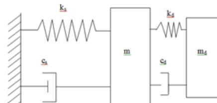
Fig. 1: The Single tuned mass damper
