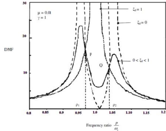
Fig. 3: Amplitude of main mass for various values of absorber damping
