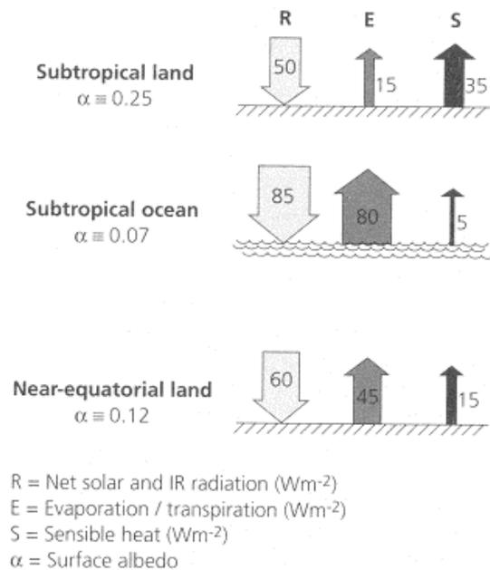
Fig. 1: Effects of three different surfaces on heat balance
